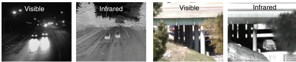
Thermal imaging cameras see in total darkness and show more scene detail.
