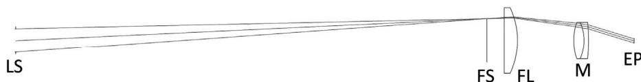
Figure 14.1 Kellner ocular at a finite distance to the lens stop. The lens stop (LS) is 8 mm in diameter. The tube length is 160 mm. The object NA is 0.025. The field stop (FS) is 15 mm in diameter. The exit pupil (EP) is 1.6 mm in diameter at an eye relief of 15.5 mm. the field of the image is 17 deg. The field lens (FL) is a standard plano-convex lens at 50 mm in focal length. The magnifier (M) is a stock doublet at 30 mm in focal length. The EFL is 25.0 mm at the d line. The angular magnification is 10X the near-point view.
